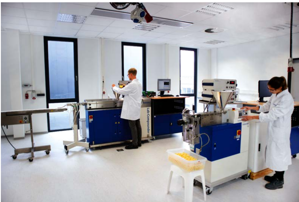
Fig. 6: Gluten-free snack products, breakfast cereals, flatbreads, pastas, purees, confectionery products, pet food, and other extruded products can be produced on a laboratory scale with Brabender single or twin screw extruders.
